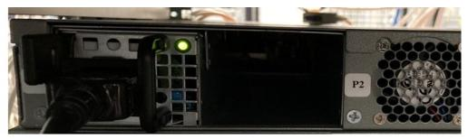
Plug the power module to the power unit as before by pushing it in. Then plug in the power cable. The current is restored, and the LED is green again.
