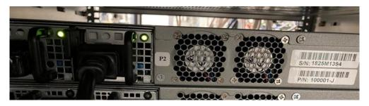
Step 4: Check the external condition of the power supply unit.
