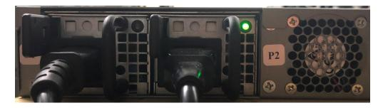
When the power cable is not plugged in to one of the power modules, the LED should be blinking red.
